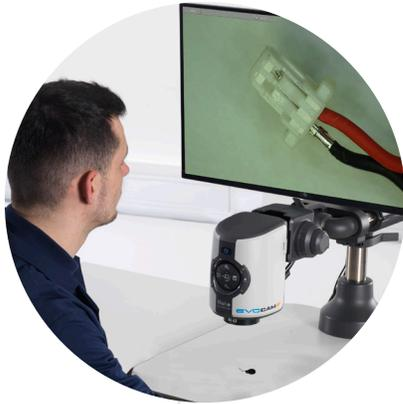
...examining the finished crimped wires through an inspection system will identify any defects and prevent faults that would occur once the wire harness is finally connected.
